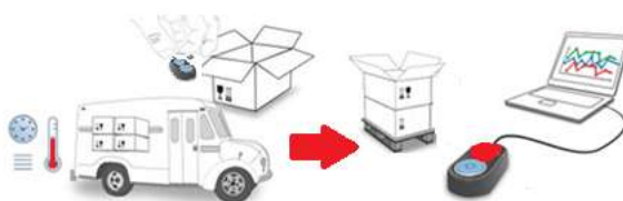
Fig. 3 – The role of the digital temperature monitoring system: from the preparation of the shipment to the successful delivery.
